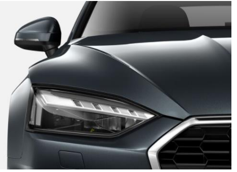
Matrix LED headlamps with Audi laser light, dynamic lighting scheme and dynamic turn signal
