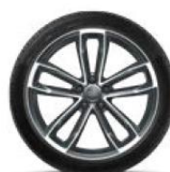
Cast aluminum wheels, 19 inch in 5-spoke Cavo design (S design), contrasting gray 8.5J x 19, 255/35 R19 tires
